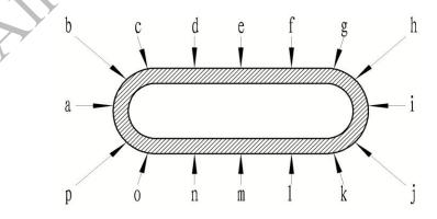
Fig.2. Method of thickness measurement
